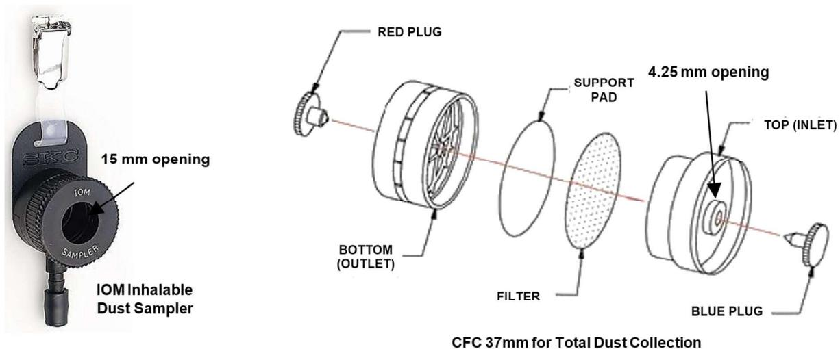
**FIG 4** – Sampling inlets of the IOM and CFC samplers.
